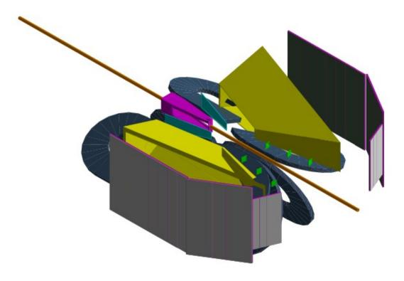
•GEM tracker•Wire chambers•Plastic scintillators•Luminosity monitor
