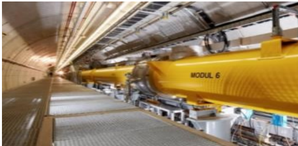
TESLA type superconducting accelerating modules 1.3 GHz
