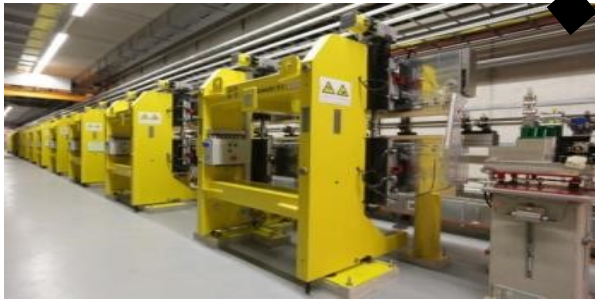
FLASH2 variable gap undulators
