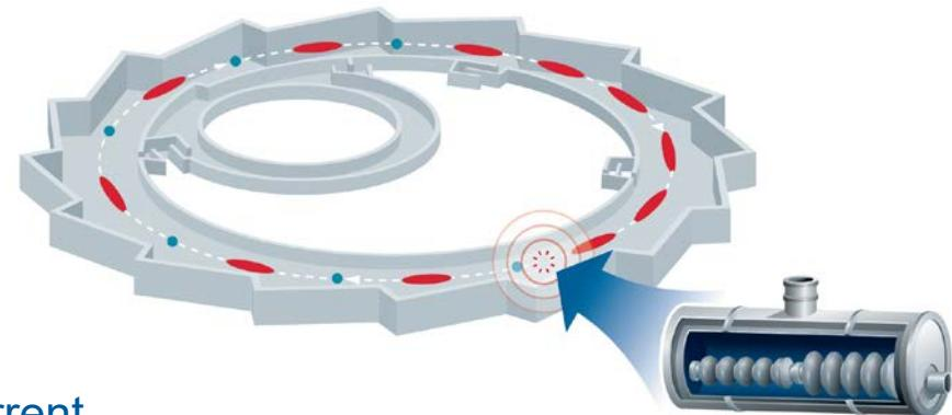
Combining two RF systems with different frequencies (1.5 GHz & 1.75 GHz) generates long and short buckets, which can be filled individually to generate optimized fill pattern.
