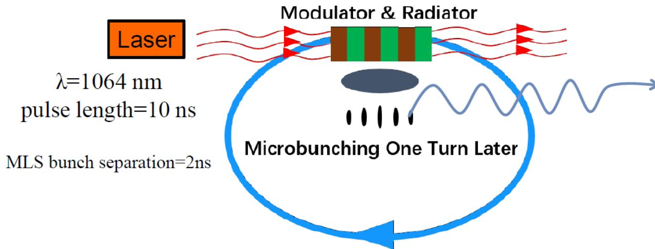
we want to proof experimentally that **micro structures** generated by a **Laser driven energy modulation** inside an undulator at a resonant wavelength of 1064 nm lead to enhanced **coherent radiation** on the same undulator **one turn** (160 ns) **later**
