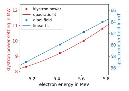
First energy measurements with dipole spectrometer in injector section
