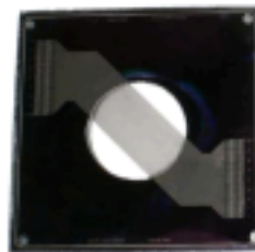
MMD: 64 strips, 100 \mu\text{m} pitch, 40 \mu\text{m} width, 1 \mu\text{m} thick
