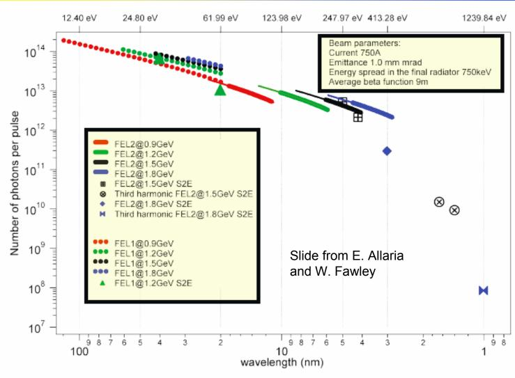
Lines predicted using M.Xie formulae for expected FERMI parameters assuming 40fs pulse length Points Ginger and Genesis simulations for S2E files
