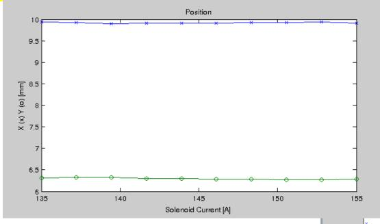
Optimizing the laser pointing (monitoring on the virtual cathode) to minimize the bunch transversal drift when scanning the gun solenoid.
