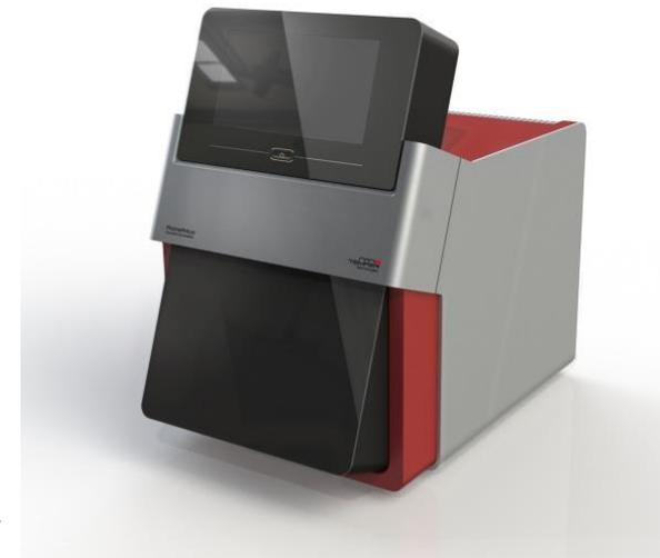
**Principle behind the nanoDSF.** Increasing temperature causes protein unfolding that can be assessed by monitoring changes of tryptophan fluorescence at 330nm and 350nm wavelength.
