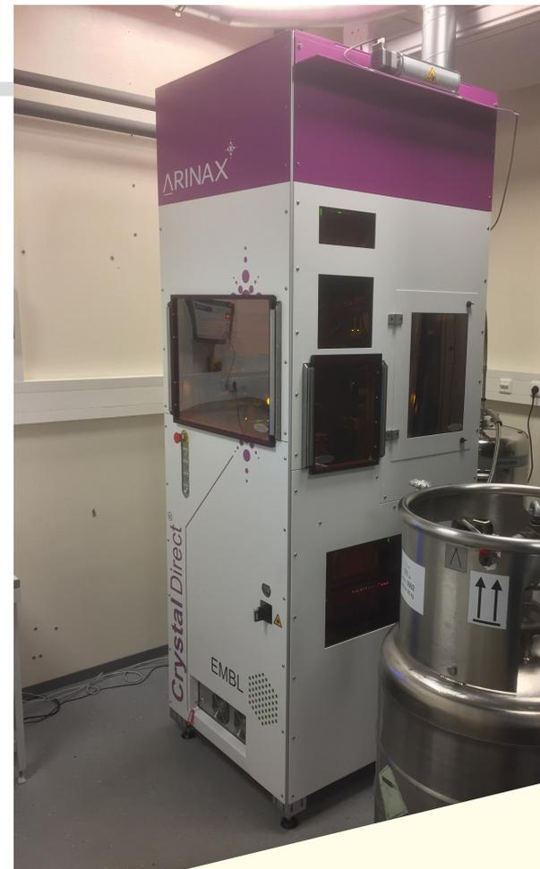
A robotic **CrystalDirect Harvester** (arinax.com) system for (remote) harvesting and cryo-cooling of crystals is operational
