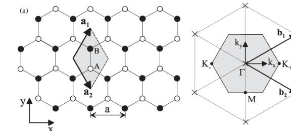
Lattice structure of graphene [4]
