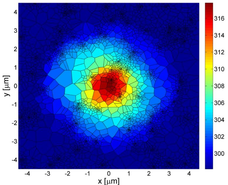
Temperature profile at steady state condition
