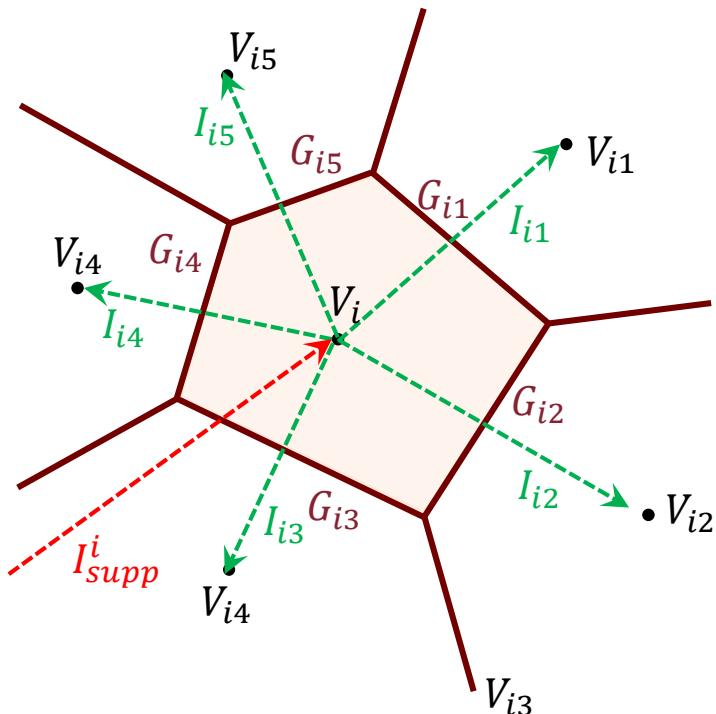
$G_{ij}$  comprises of grain resistance and GB resistance due to mismatch angle.
