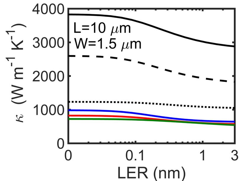
Strong width dependence of thermal conductivity in graphene ribbons arising from the dependence of normal contribution and the interplay between LER and normal scattering
