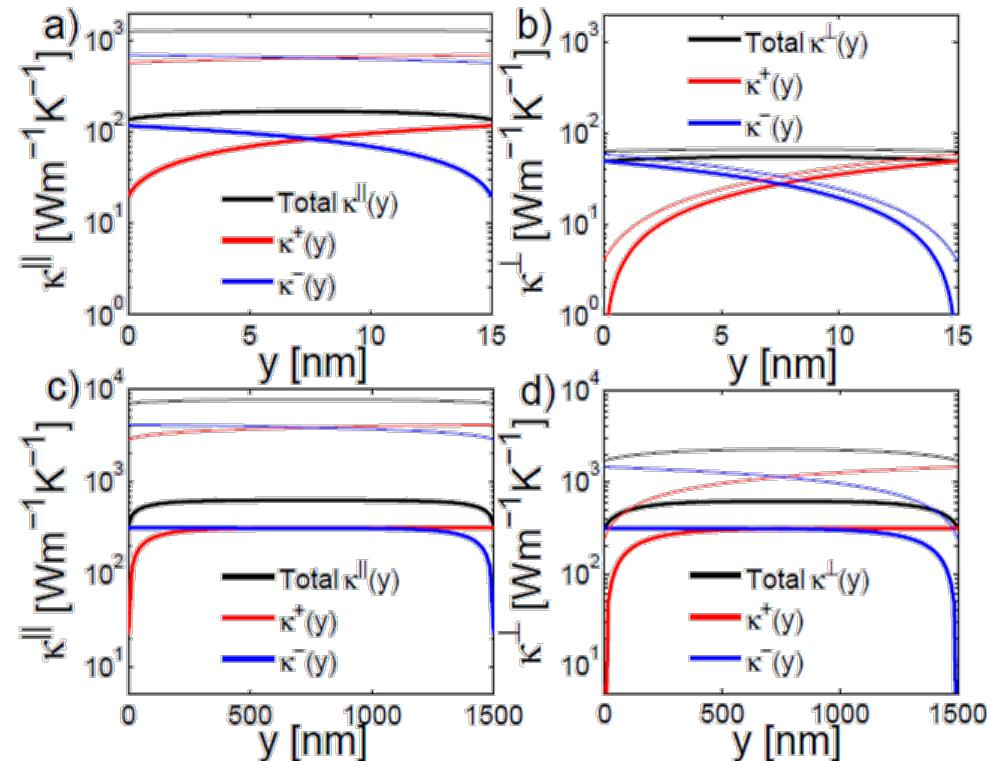
Wide versus narrow – in narrow ribbons (a,b) transport is dominated by edges and LER scattering, in wide ones (c,d) thermal transport dominated by internal (phonon-phonon)
