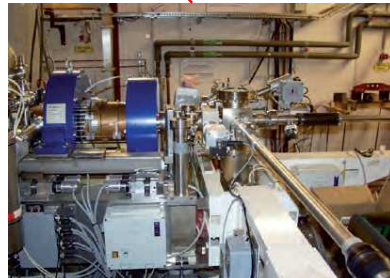
RF electron gun 5 \text{ MeV}
