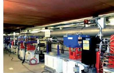
Bunch compressors 50 \text{ A} \rightarrow 2 \text{ kA}
