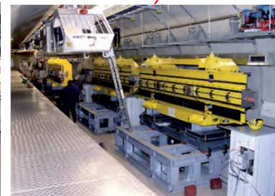
Undulator Assembly \text{NdFeB} , Length 6 \times 4.5 \text{ m} Magnetic period 27 \text{ mm} Fixed Gap 12 \text{ mm}
