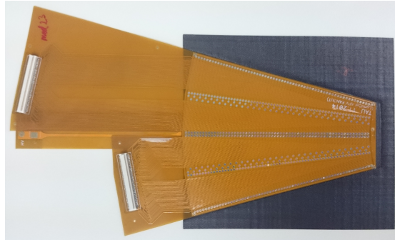
Figure 3: A thin detector plane. The black part is the carbon fibre support. The silicon sensor is covered by the Kapton fan-out which has two connectors for front-end boards.
