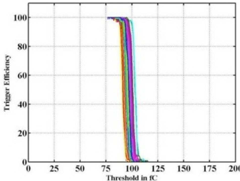
Trigger efficiency for a 100 fC signal as a function of threshold: Very homogeneous performance of all channels in a chip
