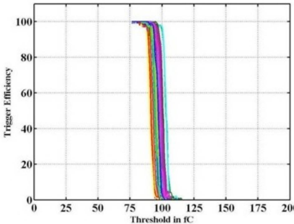
Trigger efficiency for a 100 fC signal as a function of threshold: Very homogeneous performance of all channels in a chip
