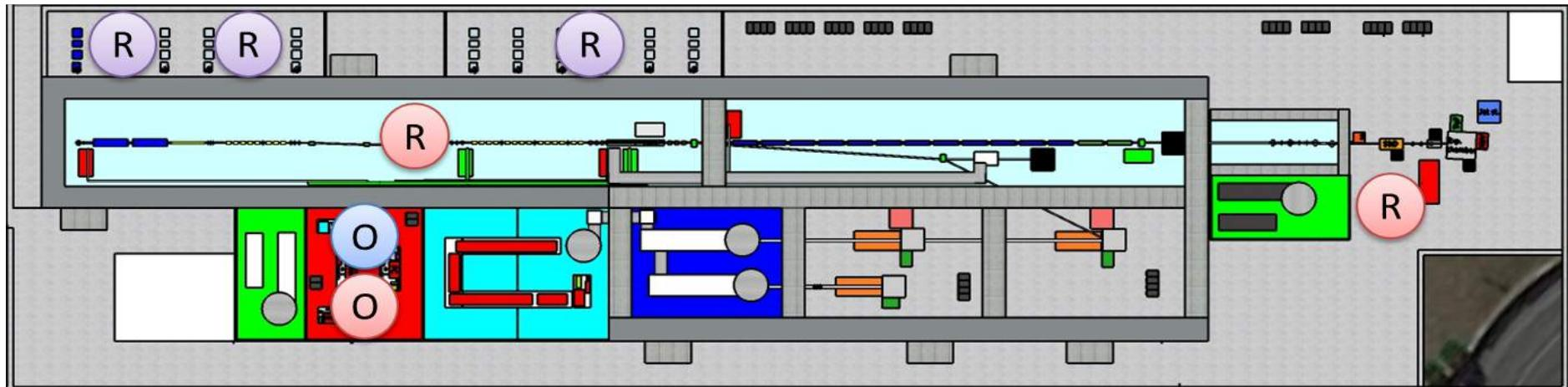
**Synchronization system:** A fine temporal alignment among all the relevant sub-system oscillators that guarantees temporal coherence of their outputs (**precision  $\sim 10\text{fs}$** )
