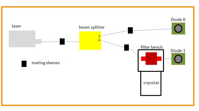
Setup for screening the laser behavior during cool-down and warm-up cycle
