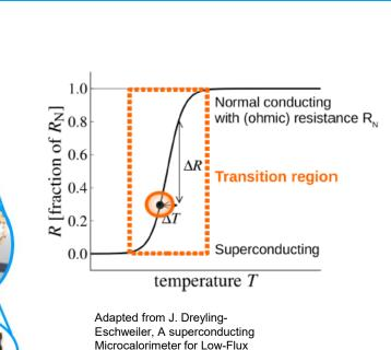
Detection of Near-Infrared Single Photons
