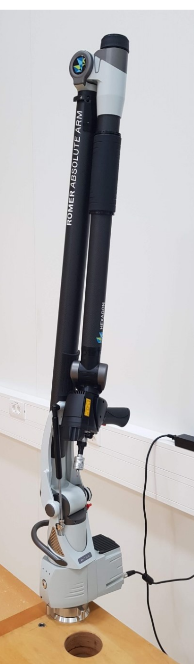
Metrology arm in DESY Laboratory
