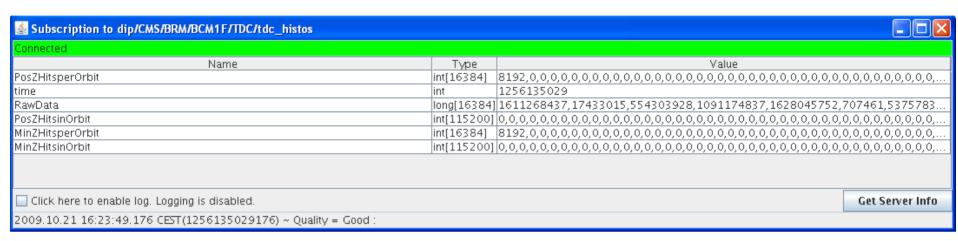
**PosZHitsperOrbit** (name to be changed to +ZHitsperOrbit)→Hits/orbit in 4 detectors of +Z side.
