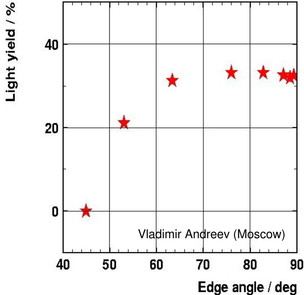
Effect of new ( $90^{\circ}$ ) vs old ( $45^{\circ}$ ) quartz plate cut on light yield with simulation package LITRANI
