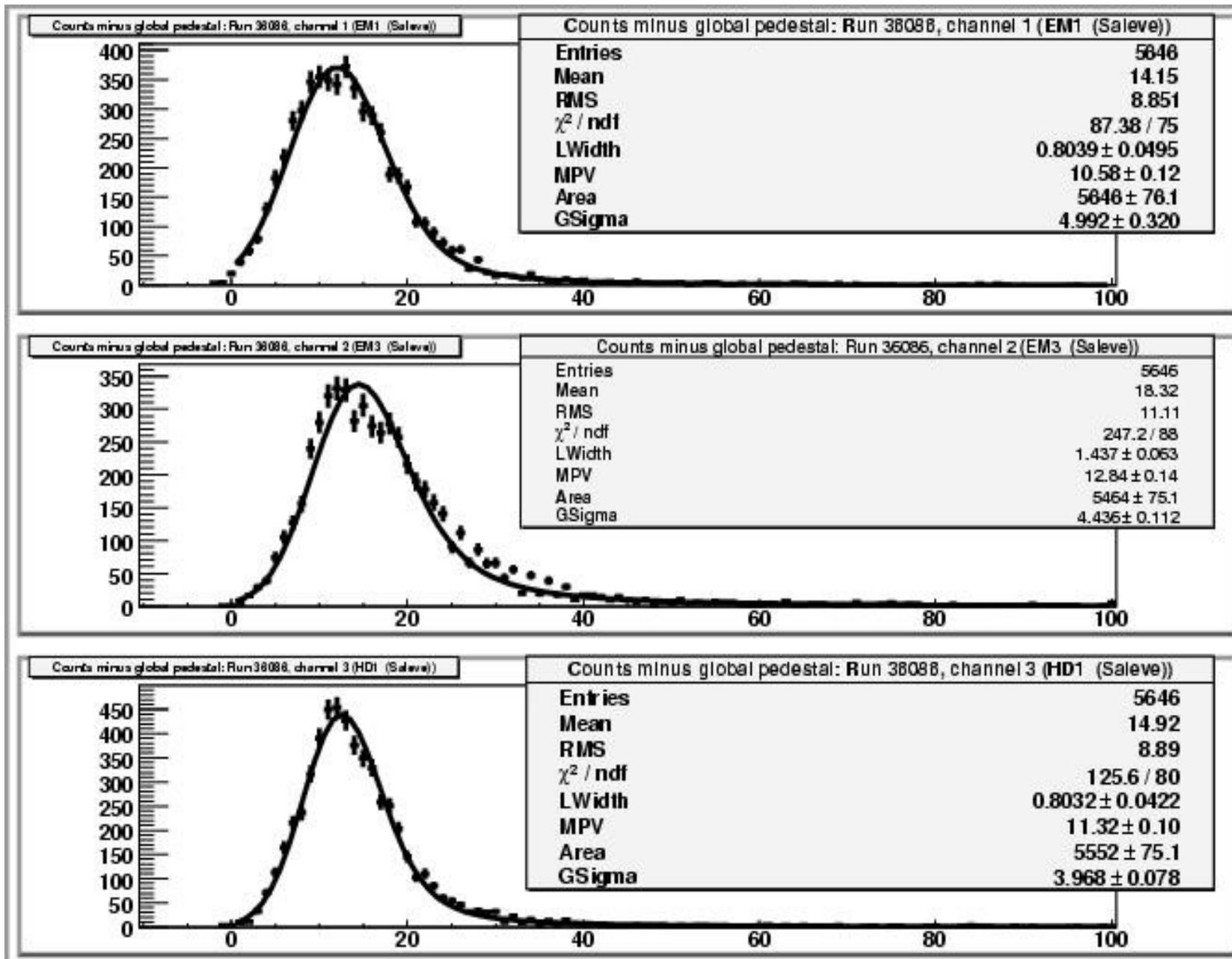
EM1, EM3, HD1 response to muons fitted with convolution of landau and gaus
