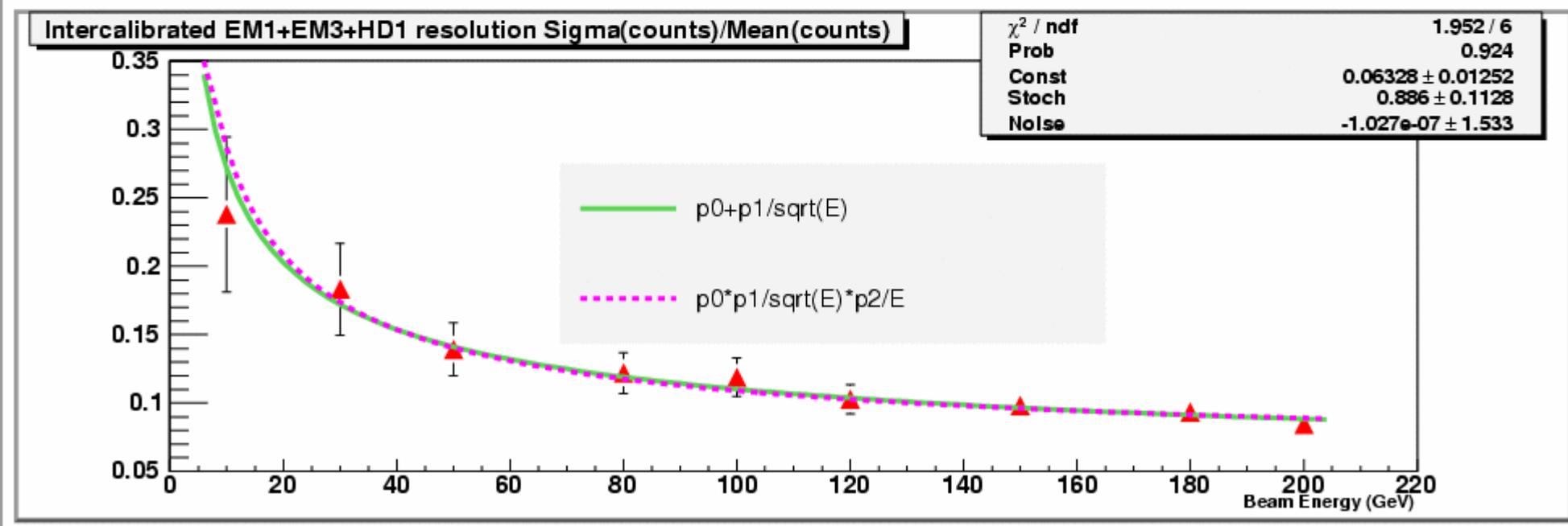
Electron energy scan results to be revisited using wire chamber info + cleaning cuts
