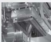
Double crystal multi- layer monochroma- tors with three stripes
