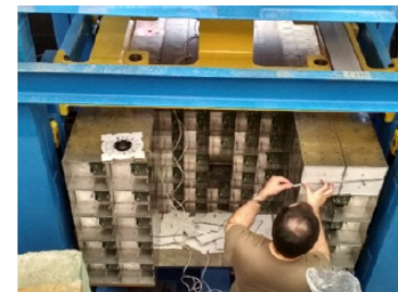
Installation of FEE on the rare side Of the FHCAL
