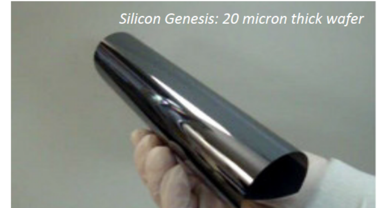
Ultra-thin chip (<50 um): flexible with good stability
