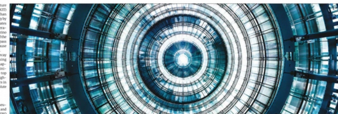
KATRIN's main spectrometer, the largest ultra-high-vacuum vessel in the world, contains a dual-layer electrode system comprising 15,000 wires to shield the inner volume from charged particles.
