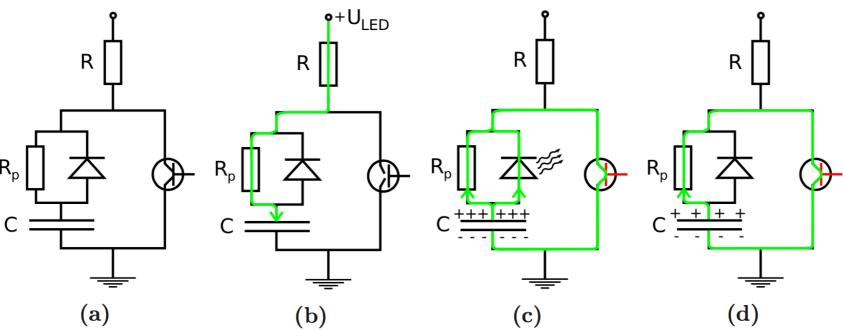
LED board creates very short light pulse for calibration/linearization of photodetectors
