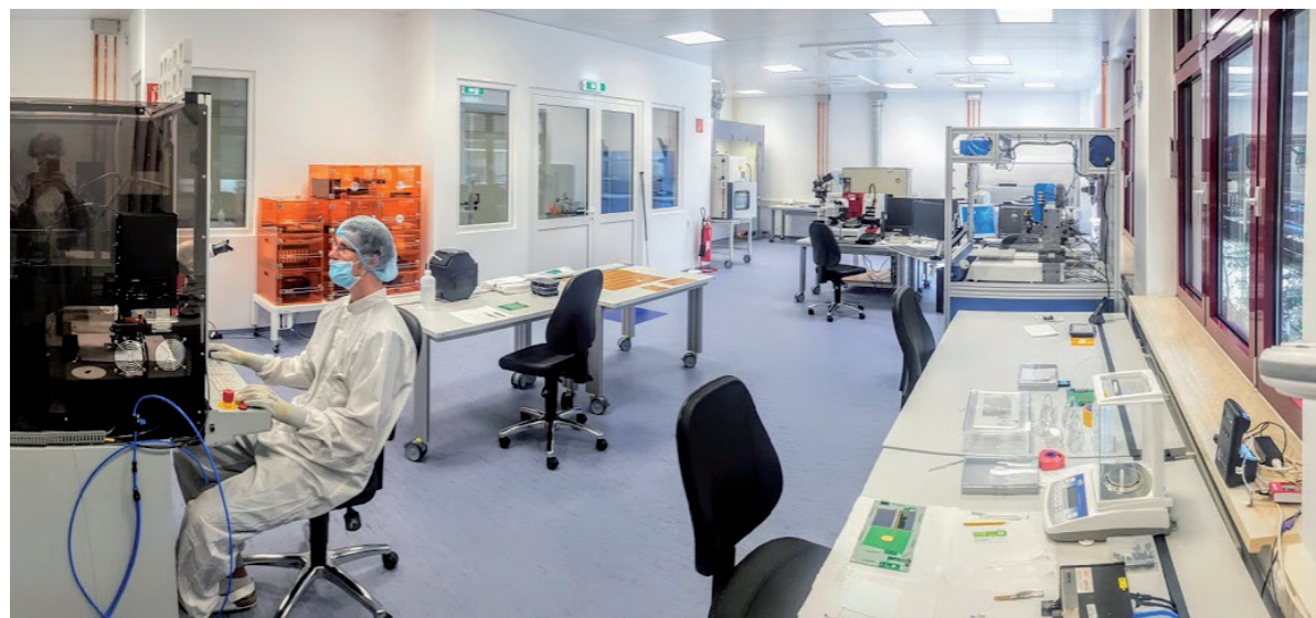
Figure 1 Cleanroom for ATLAS strip detector module construction at the DESY Zeuthen site
