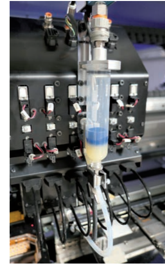
Figure 3 New dispensing tool within the SMD placement automat, with the glue cartridge in the foreground
