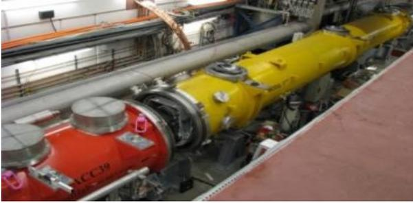
TESLA type superconducting accelerating modules 1.3 GHz
