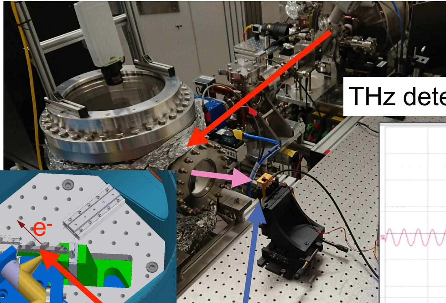
THz detector signal from transition radiation
