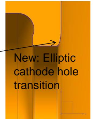
New: Elliptic cathode hole transition
