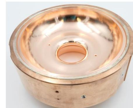
Final machined front body of Gun 5 with pick-up and symmetry holes
