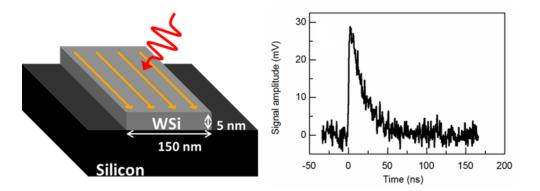
The energy absorbed by a single infrared photon is sufficient to destroy a nanowire's superconductivity and produce a transient resistance that can be seen as a voltage pulse in a constant current circuit. The right panel shows an oscilloscope trace from a single 5-micron photon.
