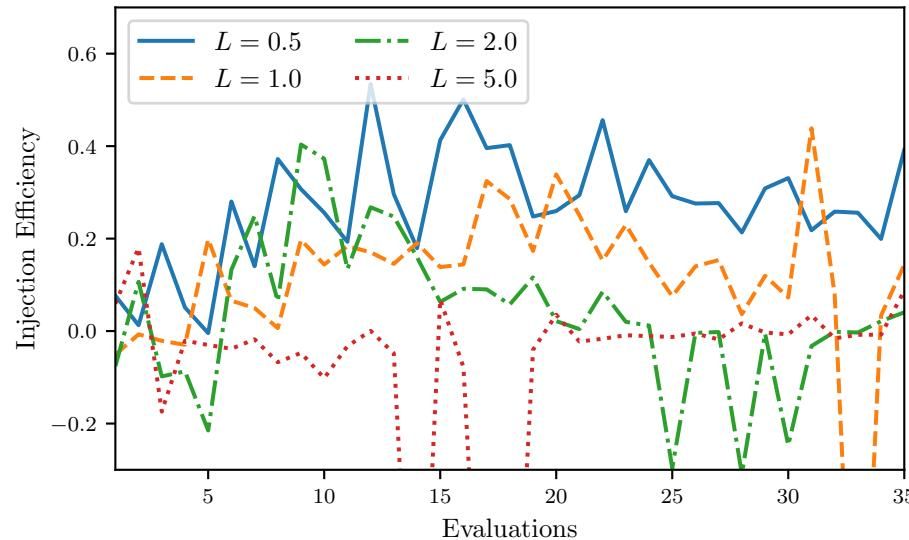
Due to the exploration behavior of GP, unaccounted beam loss can happen.
