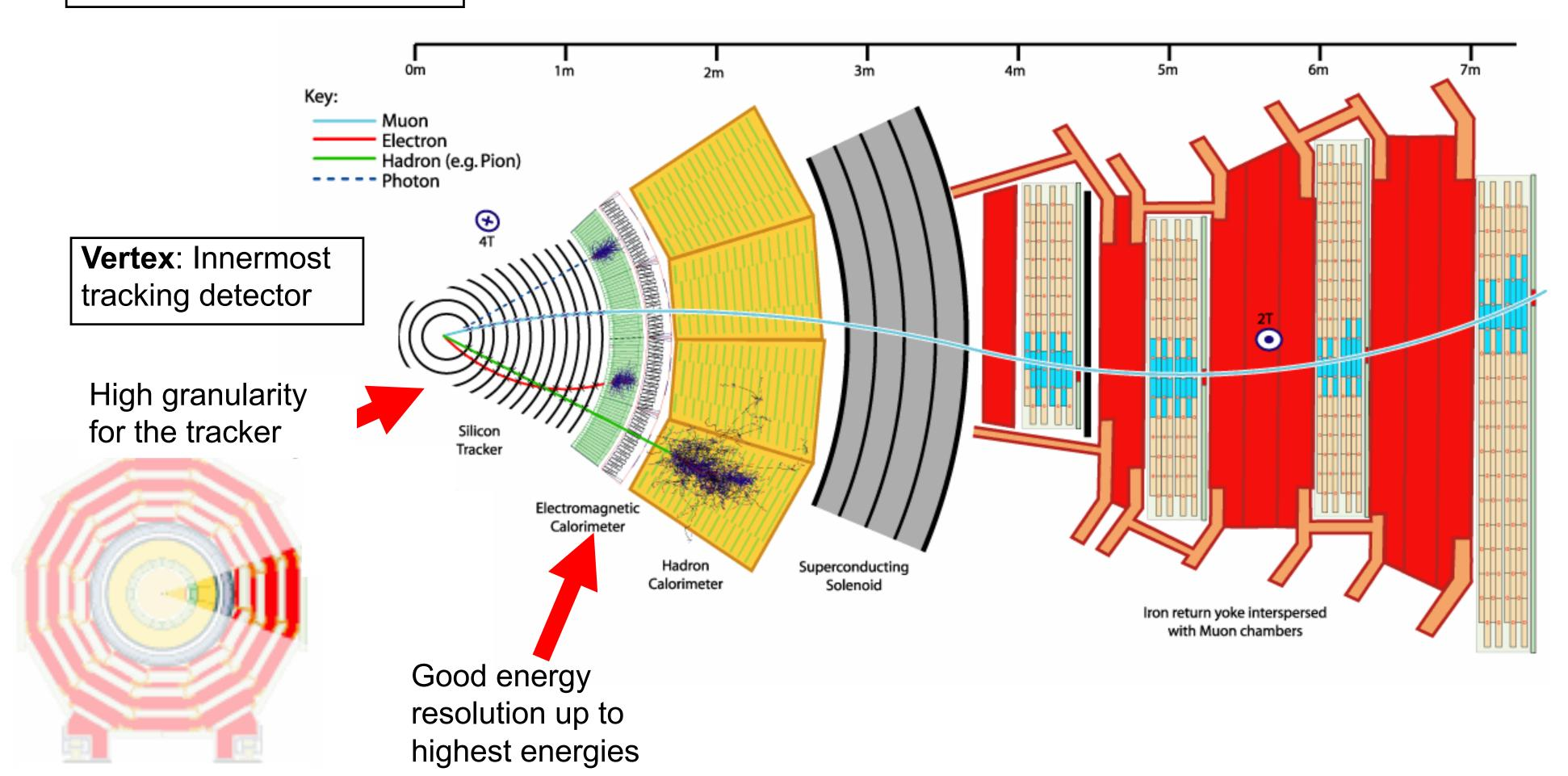
**Muon-Detectors**: Identification and precise momentum measurement of muons outside of the magnet
