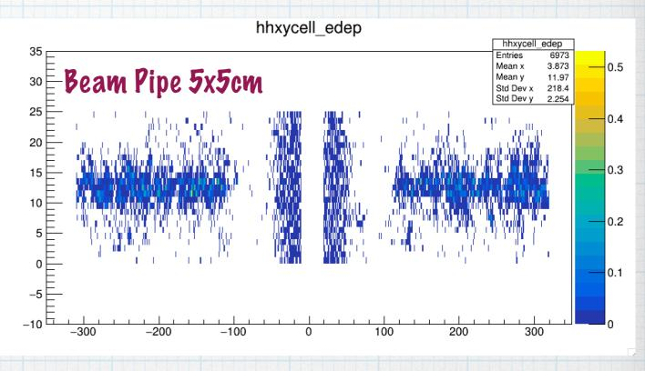
Compton MC2020 r for (xi=0.32), 16.5 GeV electrons. G4: Kapton foil of 20 um as a target, magnet 1.4T and 0.75m distance from magnet to LYSO.
