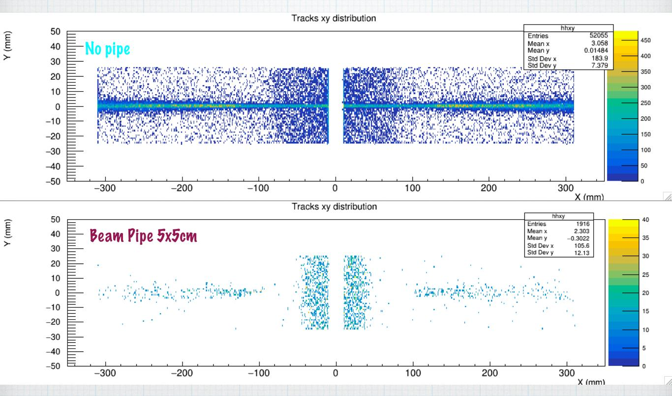
\* Big hole in the Shielding creates substantial background occupancy in LISO detectors.
