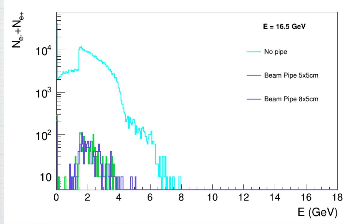
Without beam pipe we measure in Compton detectors a lot e-/e+ pairs that were created in the air. Only 4% e-/e+ come from the Target
