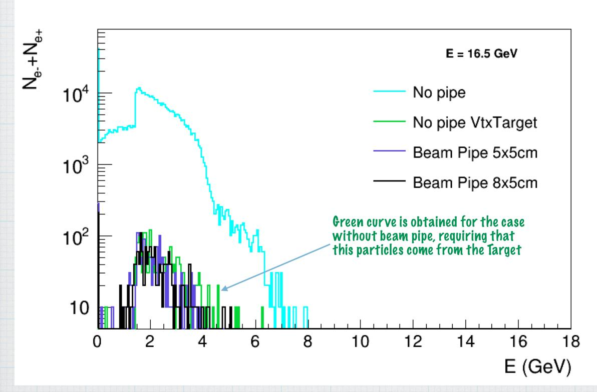
Without beam pipe we measure in Compton detectors a lot e-/e+ pairs that were created in the air. Only 4% e-/e+ are generated in the Target
