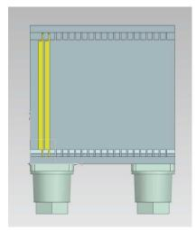
20 W absorber plates of 3.5 mm thickness, interspersed with silicon sensors encapsulated in C-fiber structures and Kapton flexible PCB for signal transport and HV supply
