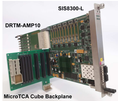
SIS8300-L and DRTM-AMP10 Gamma spectroscopy firmware
