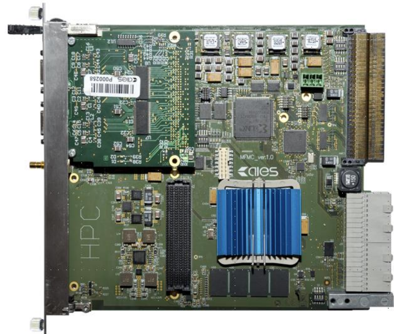
The MFMC carrier board with two FMC modules (Xilinx Artix XC7A200T)
