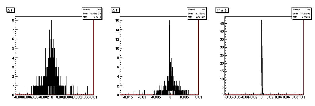
Different track selecting probably only effecting modules that are not aligned and thus remain at starting position (tails)
