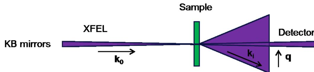
Forward-scattering fixed-target setup (FFT)
