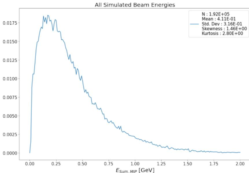
Total energy spectrum for sum of cut MIP hits, event by event. Theoretical value for Bethe-Bloch energy loss in iron should be  $\sim 0.18$  GeV
