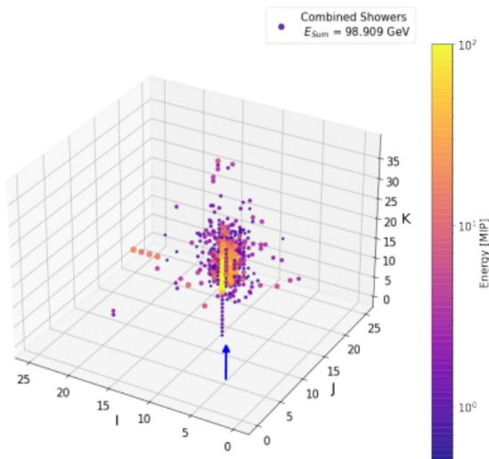
Example event display of a 80 GeV negative pion detected by the AHCAL
