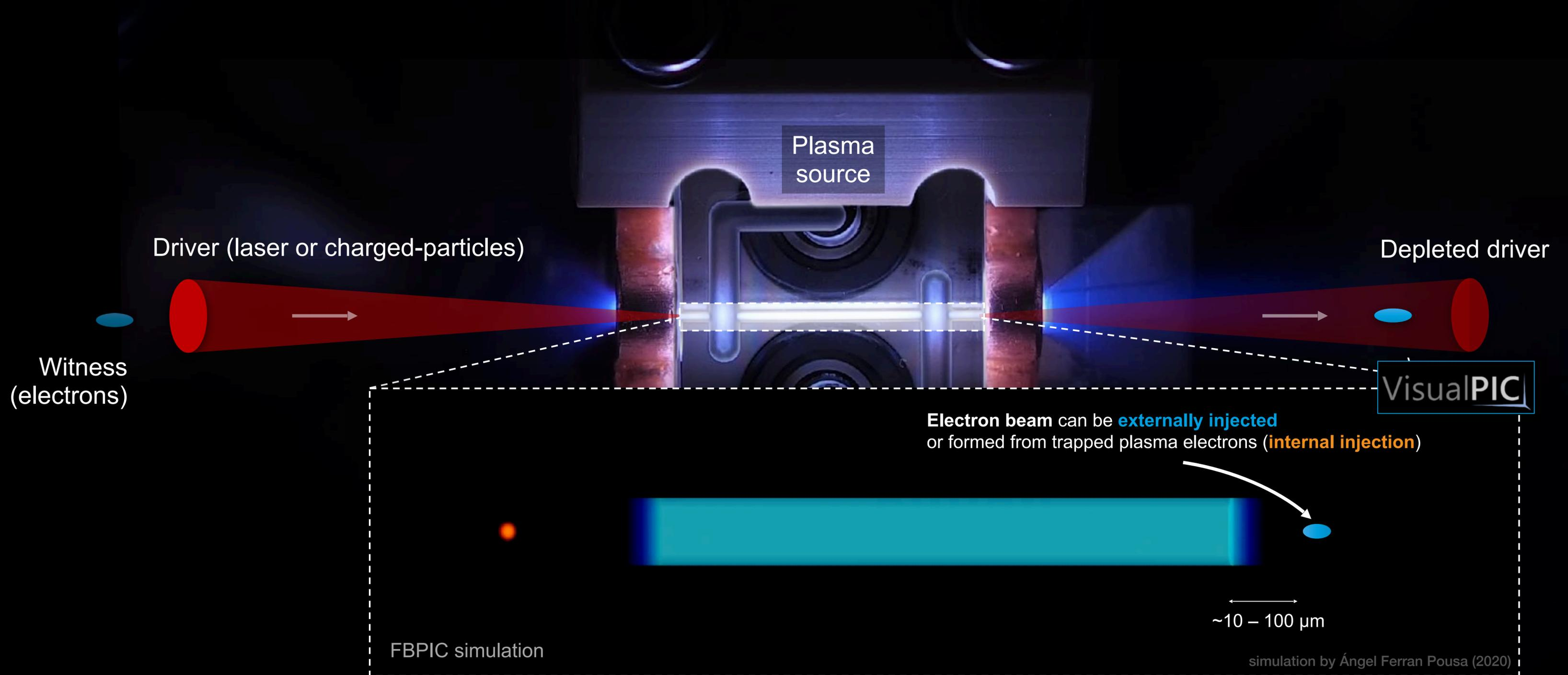
**Plasma wakefields** can sustain accelerating fields of up to **~1-100 GV/m** with focusing gradients above **~1 MT/m**
