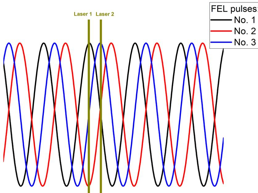
FEL phase can be determined by using two laser pulses;
