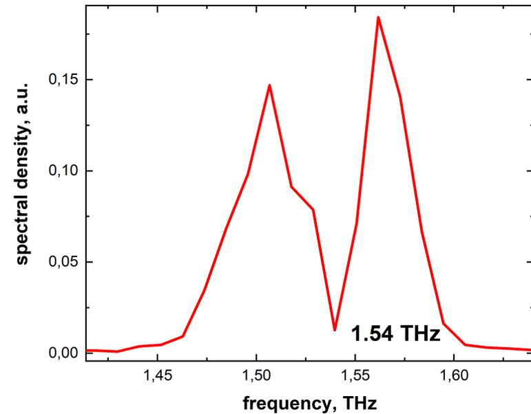
Dip in the frequency corresponds to water absorption line (1.542 THz)
