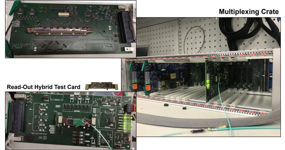
Dedicated firmware block developed for MUX Crate control and electrical tests of single components
