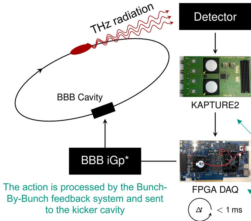
The action is processed by the Bunch-By-Bunch feedback system and sent to the kicker cavity
