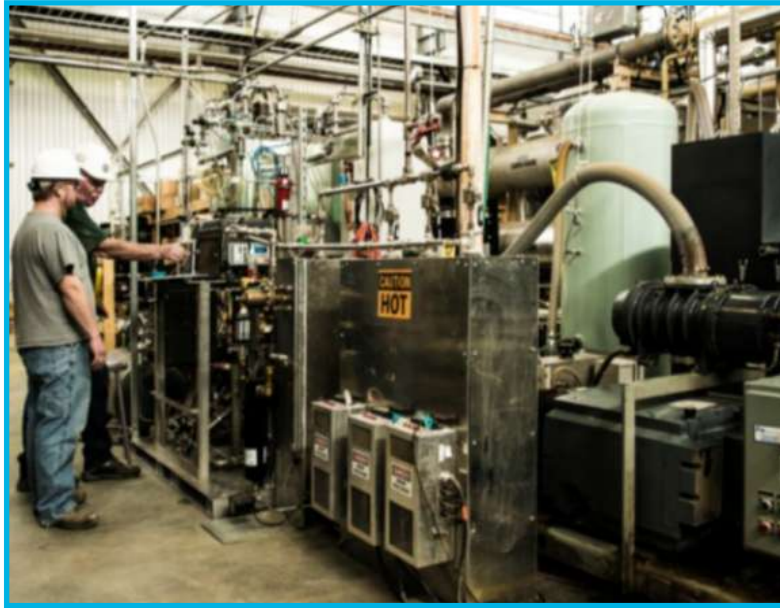
Urania - Argon extraction and purification plant in Cortez, Colorado. Capable to provide 330 kg/d of UAr with a 99.99% purity.
