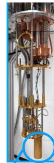
Internal structure of the dilution refrigerator
