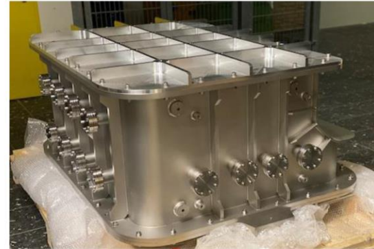
Central vacuum tank
