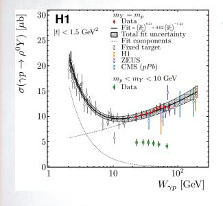
• Parametrization and fit — • this measurement:  $\sigma \propto W^{\delta}$ :  $(20 < W_{\gamma p} < 80 \text{ GeV})$   $\rightarrow$  fit elastic & dissociative together  $\delta_{el} = +0.171 \pm 0.009 \stackrel{+0.039}{-0.026}$   $\delta_{pd} = -0.156 \pm 0.026 \stackrel{+0.081}{-0.079}$ •  $\delta_{pd} \neq \delta_{el}$ :  $\rightarrow$  phasespace shaping by  $m_Y < 10 \text{ GeV cut!}$  $\rightarrow$  suppresses high  $W_{\gamma p}$  stronger than low  $W_{\gamma p}$
