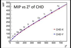
Non linear response to  $Z^2$  due to  $\checkmark$  the quenching effect in the scintillators is corrected using a "halo" model.
