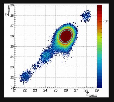
Iron events are selected within an ellipse centered at Z = 26, with 1.25  $\sigma_x$  and 1.25  $\sigma_y$  wide semiaxes for  $Z_{CHDX}$  and  $Z_{CHDY}$ , respectively, and rotated clockwise by 45°
