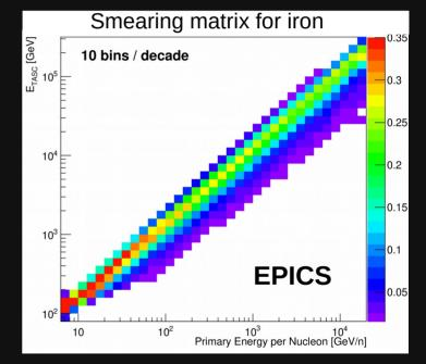
The smearing matrix is computed using Epics MC. The unfolding is performed by an iterative method based on the Bayes theorem.
