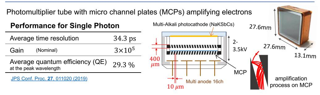
Waveform readout modules with 2.7 GSample/s on 8192 channelsAverage time resolution: 27.6 psNIM A 941, 162342 (2019)
