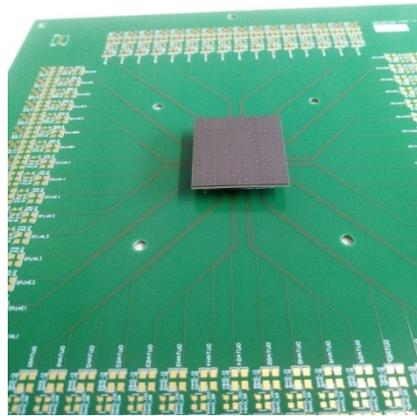
SiPM-amplifier coupling PCB
