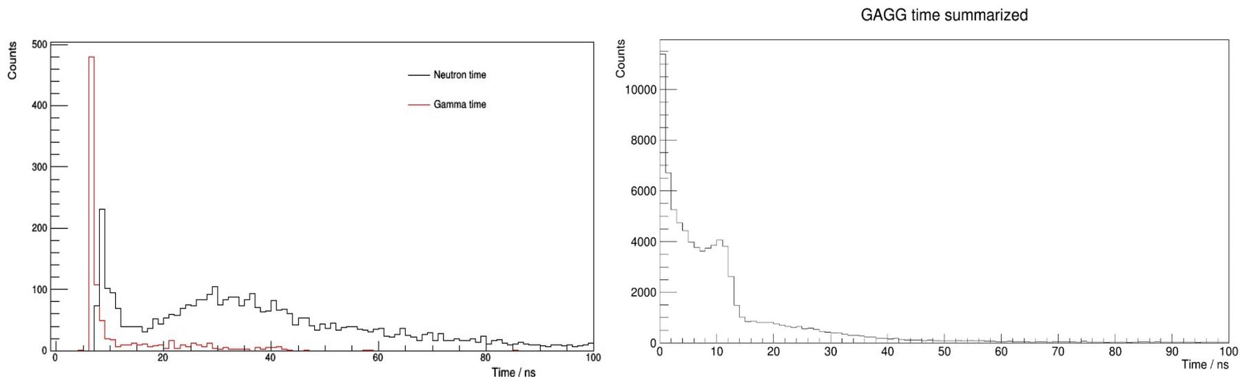
**Time spectrum of neutrons and gamma-quanta recorded with GAGG detector, according to the simulation results (left) and the measured spectrum by the STOP(matrix) channel (right)**
