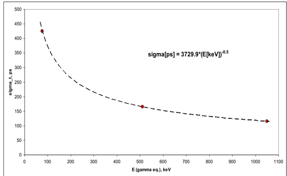
Time resolution is expected to be below 500 ps at the detection of the gamma-quanta with energy  $\sim 100$  keV, which are created by neutrons
