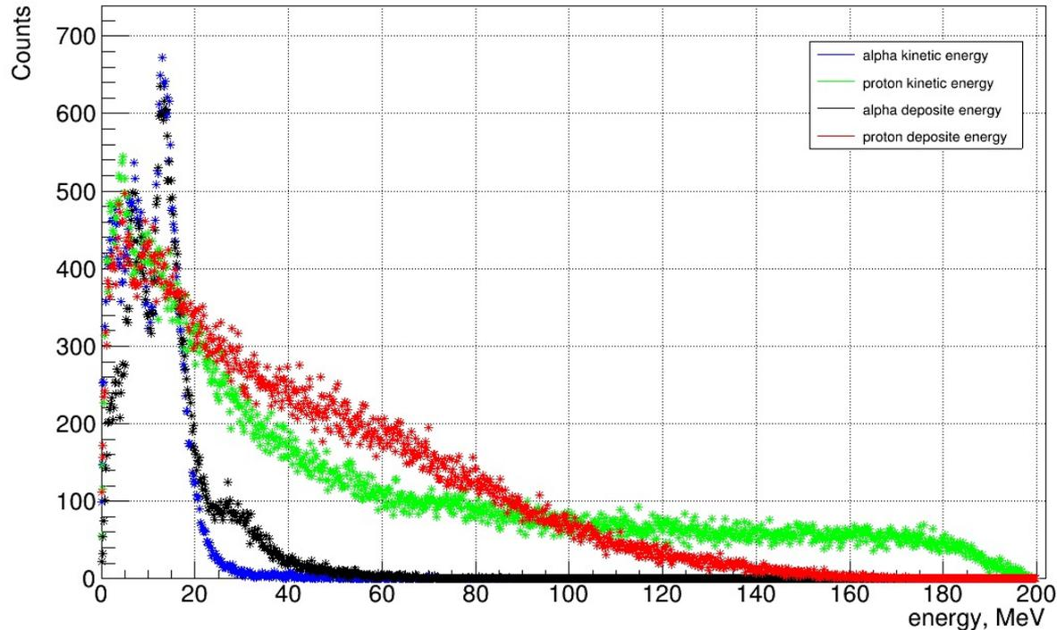
Comparison of energy distribution and energy deposition from charged particles (protons and alpha-particles) created in GAGG under 200 MeV neutrons.
