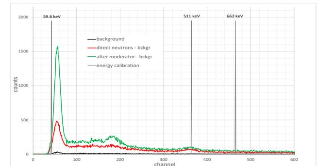
GAGG/SiPM response to Pu-Be neutron source
