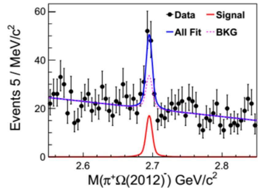
$$\frac{Br(\Omega_c^0 \rightarrow \pi^+ \Omega(2012)^-) \times Br(\Omega(2012)^- \rightarrow (\bar{K}\Xi)^-)}{Br(\Omega_c^0 \rightarrow \pi^+ \Omega^-)}$$
