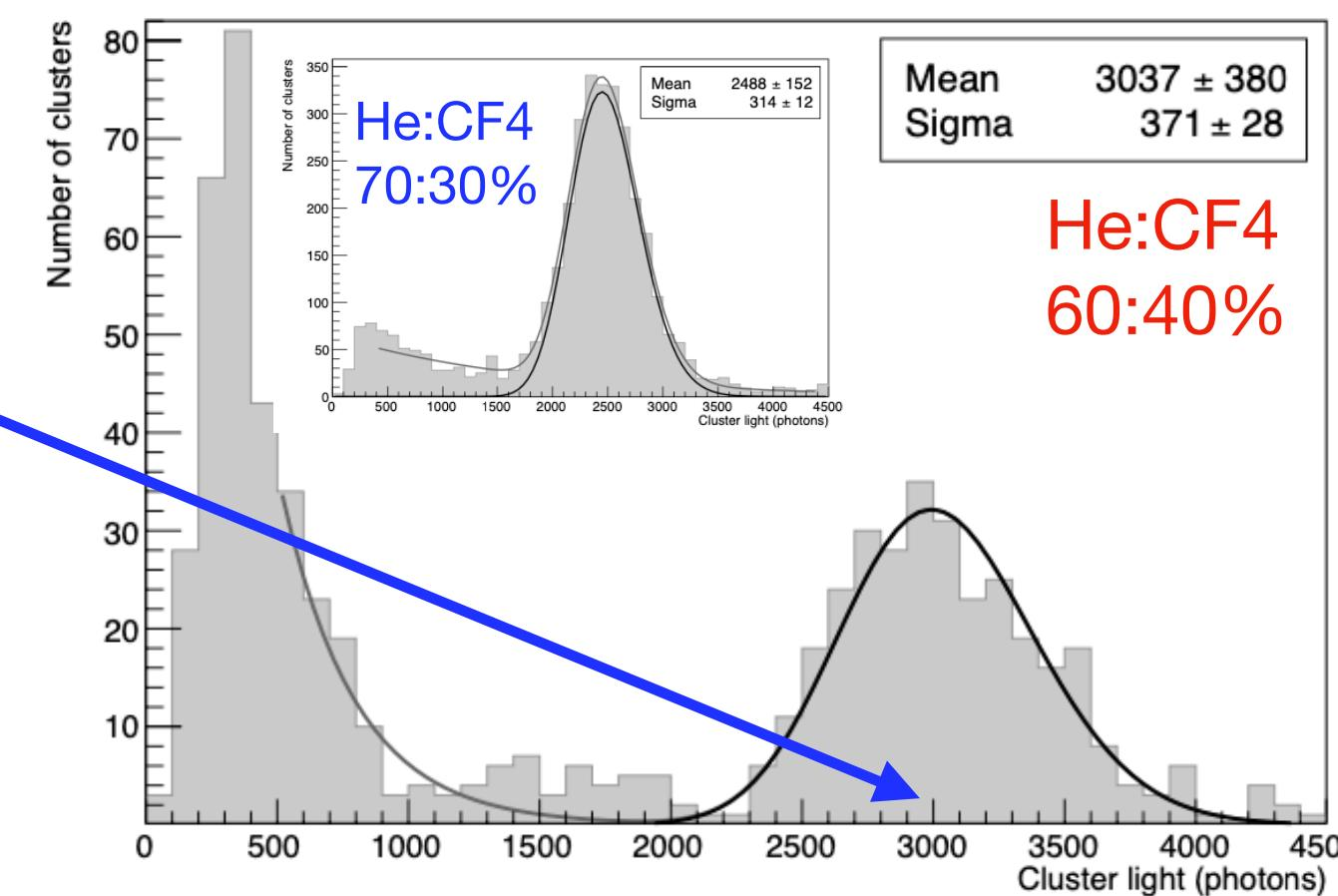
Energy resolution of 15% at 5.9 keV<sub>ee</sub> with sCMOS and PMT
