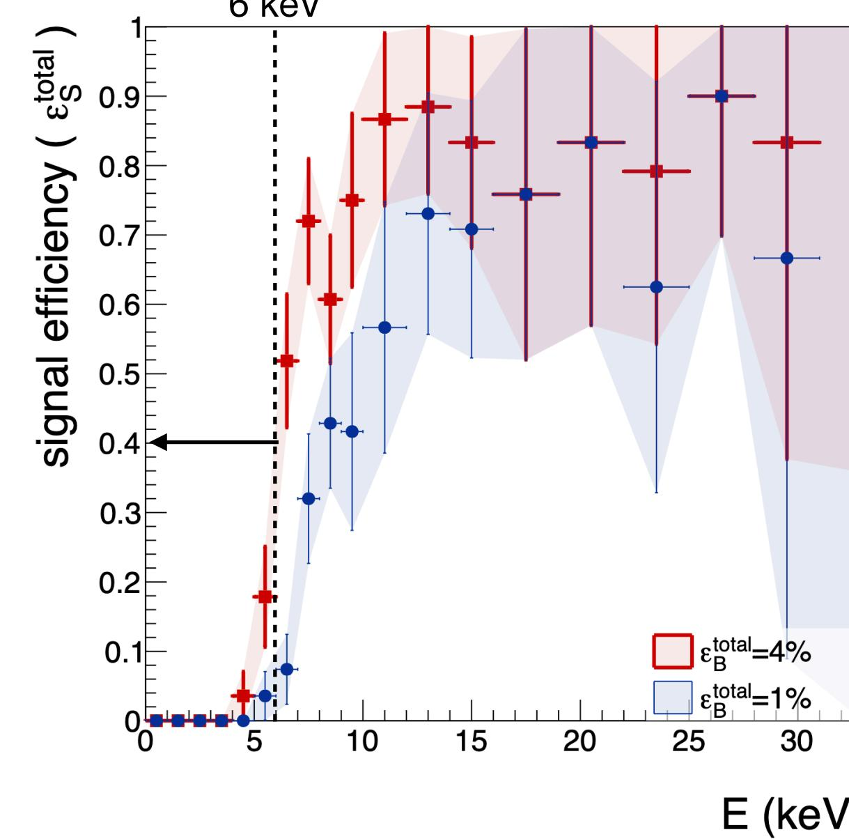
**40% nuclear recoil efficiency at 6 keV<sub>ee</sub>
