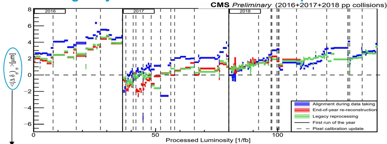
Mean difference in  $\phi$  residuals for modules overlapping in the  $\phi$  direction in the barrel pixel
