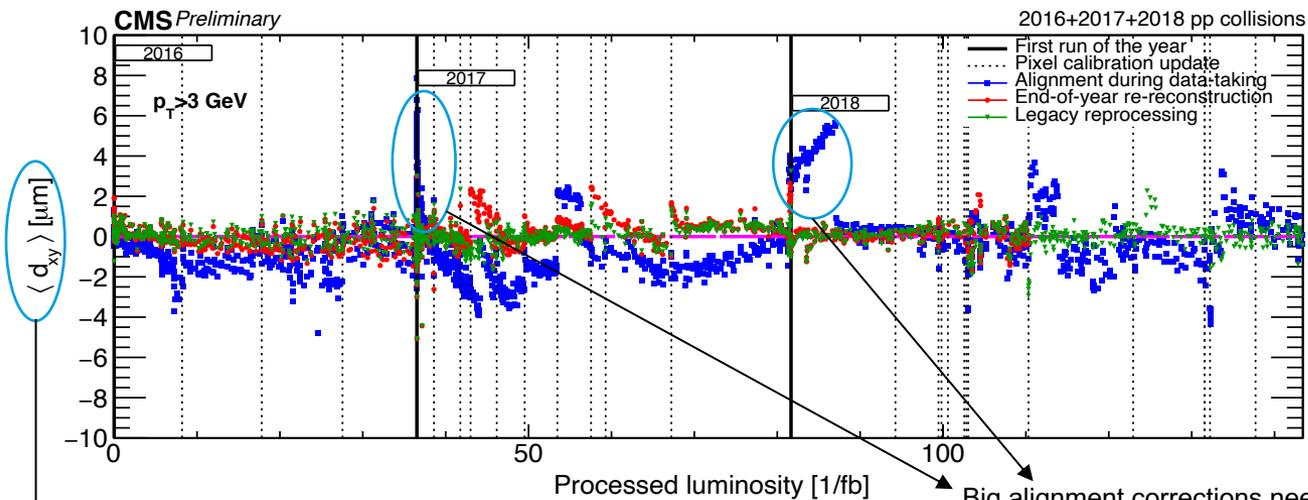
Mean distance in the transverse plane of the tracks at their point of closest approach to a refit unbiased primary vertex
