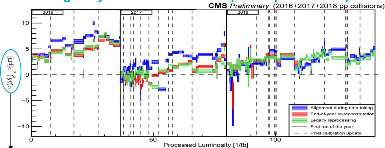
Mean difference in  $\phi$  residuals for modules overlapping in the  $z$ -direction in the barrel pixel
