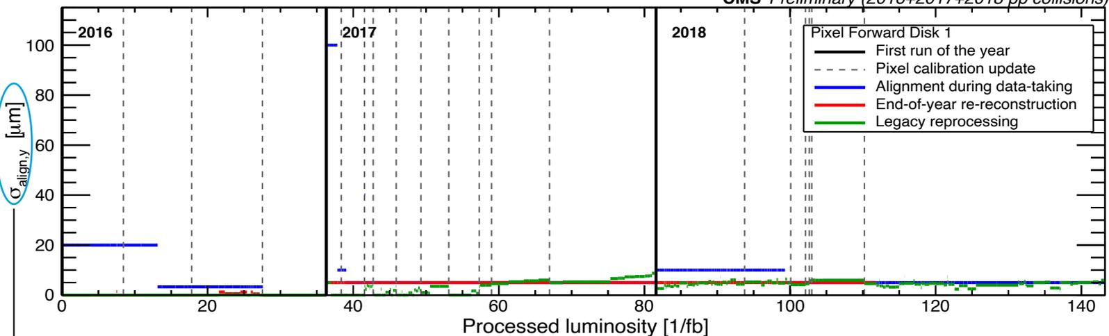
Contribution from the misalignment of the sensors to the total hit resolution for the outer ladders of the first pixel barrel layer and the first disk of the forward pixel in local  $y$ -direction
