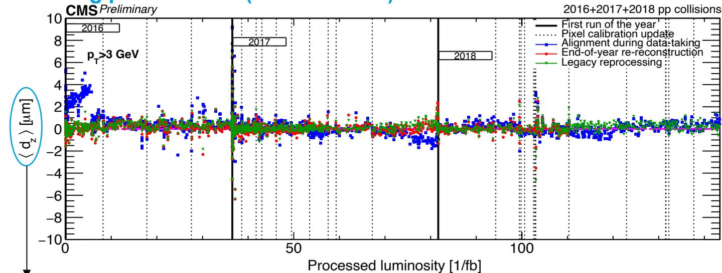
Mean distance in the longitudinal plane of the tracks at their point of closest approach to a refit unbiased primary vertex
