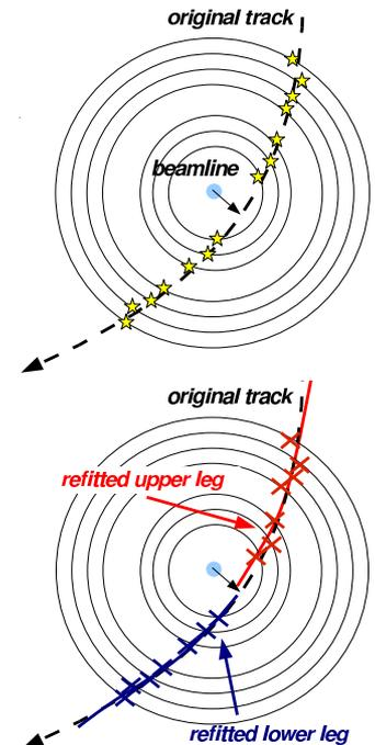
Difference of transverse impact parameter between the two halves of cosmic tracks split at their point of closest approach to the interaction region
