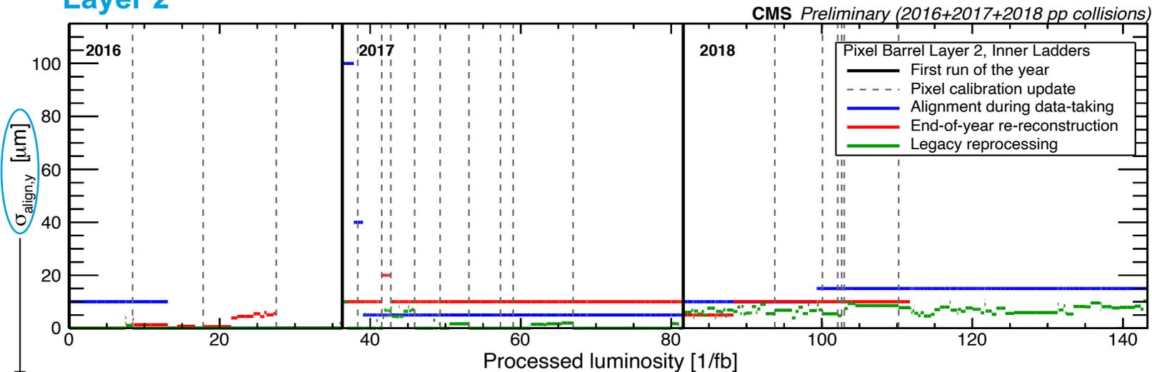
Contribution from the misalignment of the sensors to the total hit resolution for the inner ladders of the first and second pixel barrel layer in local y-direction
