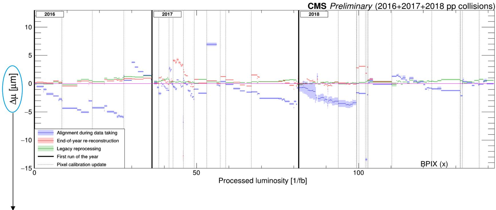
>  $\Delta\mu$ : indicator of residual bias due to accumulated effects from radiation in the silicon sensors
