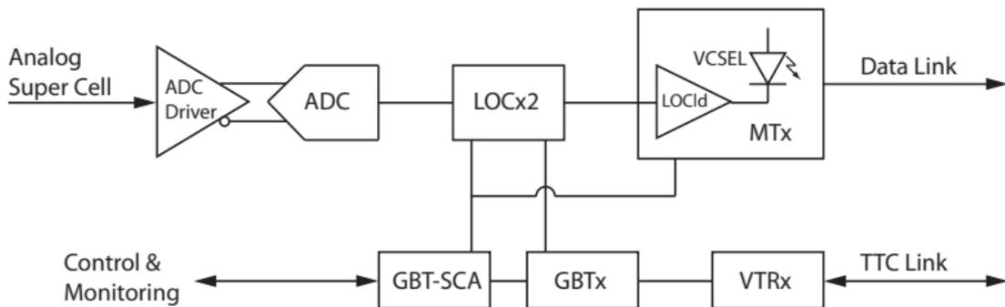
LTDB digital section includes two signal flow paths: the data link and the control (TTC) link.
