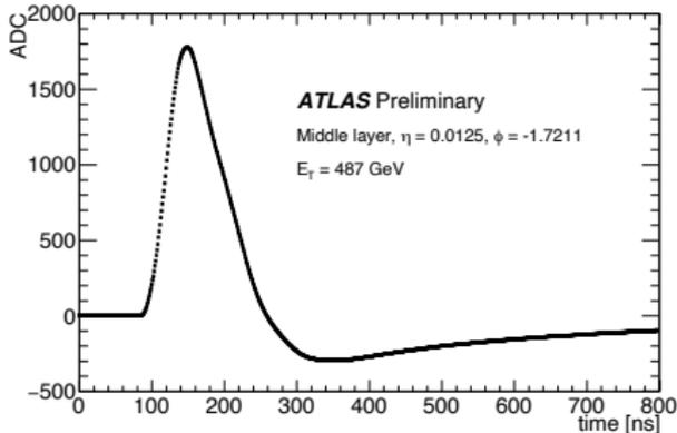
Amplitude pulse vs injected calibration signal
