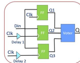
**Triple Module Redundancy with temporal delay**
