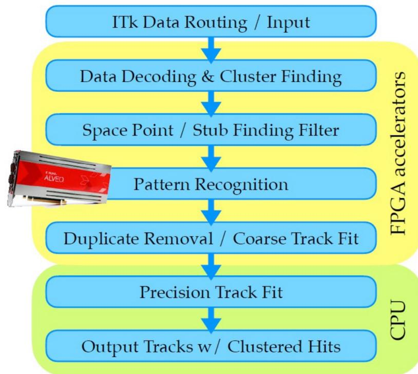
**Example of commodity-based solution for track reconstruction at the Event Filter Trigger**
