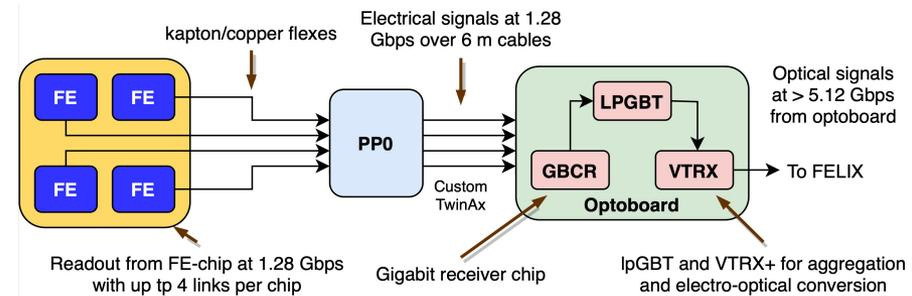
ITk pixel on-detector data transmission chain
