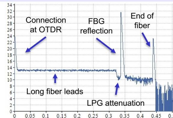
**OTDR measurement of LPG + FBG fiber optic sensors**
